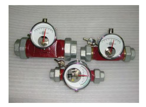
**HNMS** or **HNMQ** oscillating flap system **not tight sealing**, for pure, liquid and also aggressive substances, up to **80** ° **C**, 20 ° E, inasfar as GBz, WBz, Rg, Ms, PP are resistant. ND 10/16 at least **0.5** bar constant pressure.
